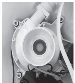
14. Replace waste pump
